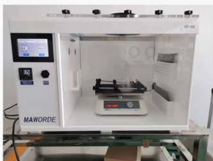
Integration of Shaker into Anaerobic Enclosure
