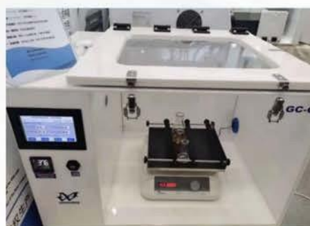
Integration of Shaker into Anaerobic Enclosure
